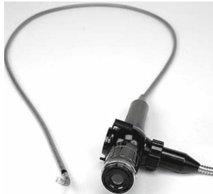
Fig. 1. Example of flexible endoscope
