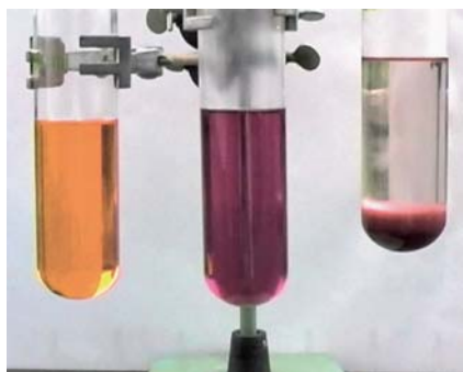
Figure 12.1 Self-immobilization of a homogeneous metallocene catalyst with ethylene in a Schlenk tube. Left: a solution of the catalyst precursor in toluene (yellow). Center: after activation with methylaluminoxane (red). Right: the precipitated self-immobilized catalyst (dark red) [2].
