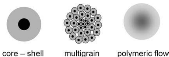
Figure 3.1 The basic particle morphology as assumed in core-shell, multigrain, and polymeric flow models.
