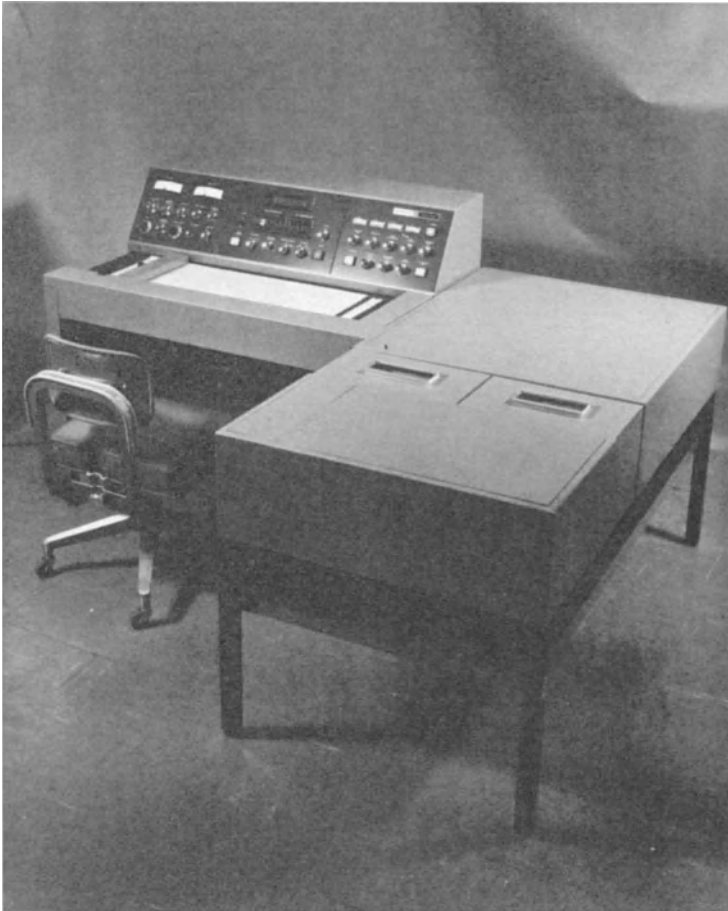
Fig. 2-20. The Perkin-Elmer Model 180 infrared spectrophotometer. (Courtesy of Perkin-Elmer Corp., Norwalk, Conn.)
