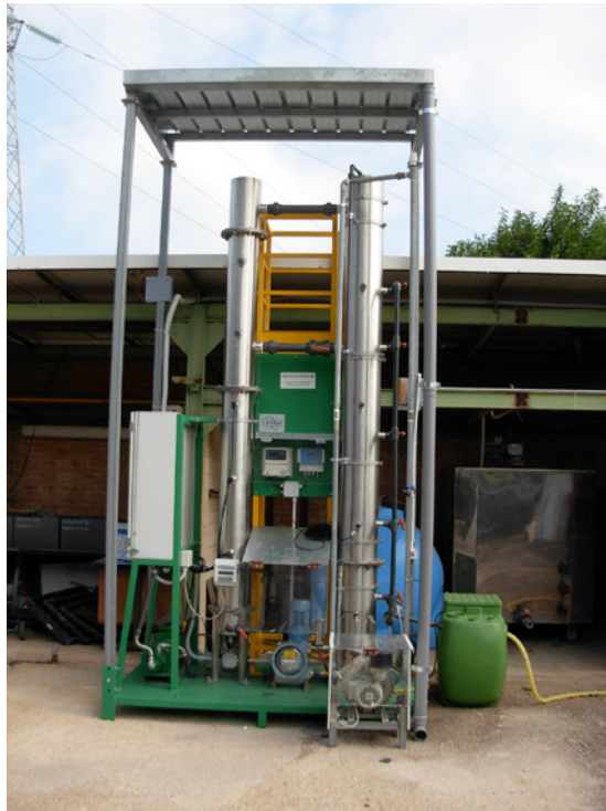
Figure 6.1 Picture of SBBGR pilot plant.
