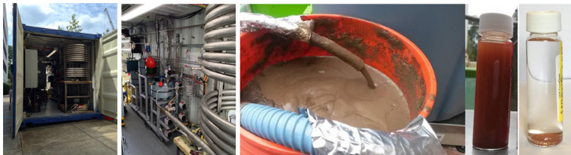
Figure 15.7 Pictures of the SCWO container unit at Duke University prior to installing thermal insulation. The system is designed to handle the fecal waste of about 1000–1500 people. On the right, pictures of a typical slurry experiment with the slurry feed (4.3% biosolids, 9% IPA (center)). Treated effluent (right), and after gravity settling (far right). The final effluent is odourless.
