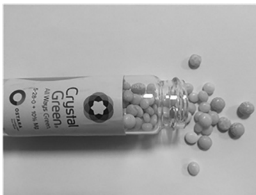
Figure 17.8 Picture of the Crystal Green struvite produced by the Pearl process developed by Ostar.
