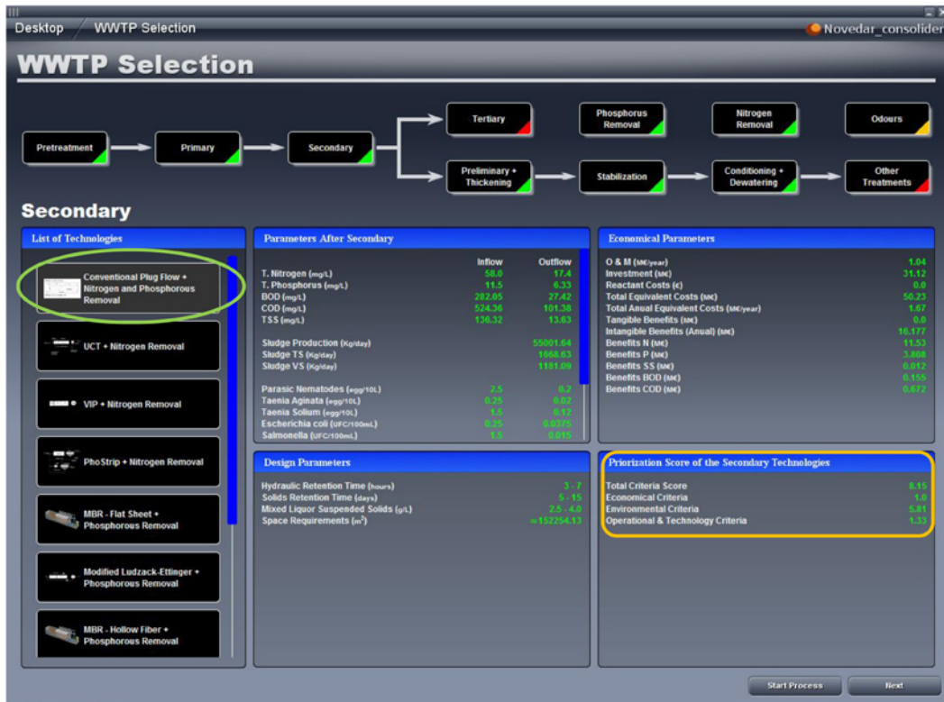
Figure 26.6 EDSS screen with the list of feasible secondary treatment alternatives for case study#1, when influent flow rate is 20% higher than the real value. The score for the best ranked alternative is presented for the economic, environmental and operational criteria.
