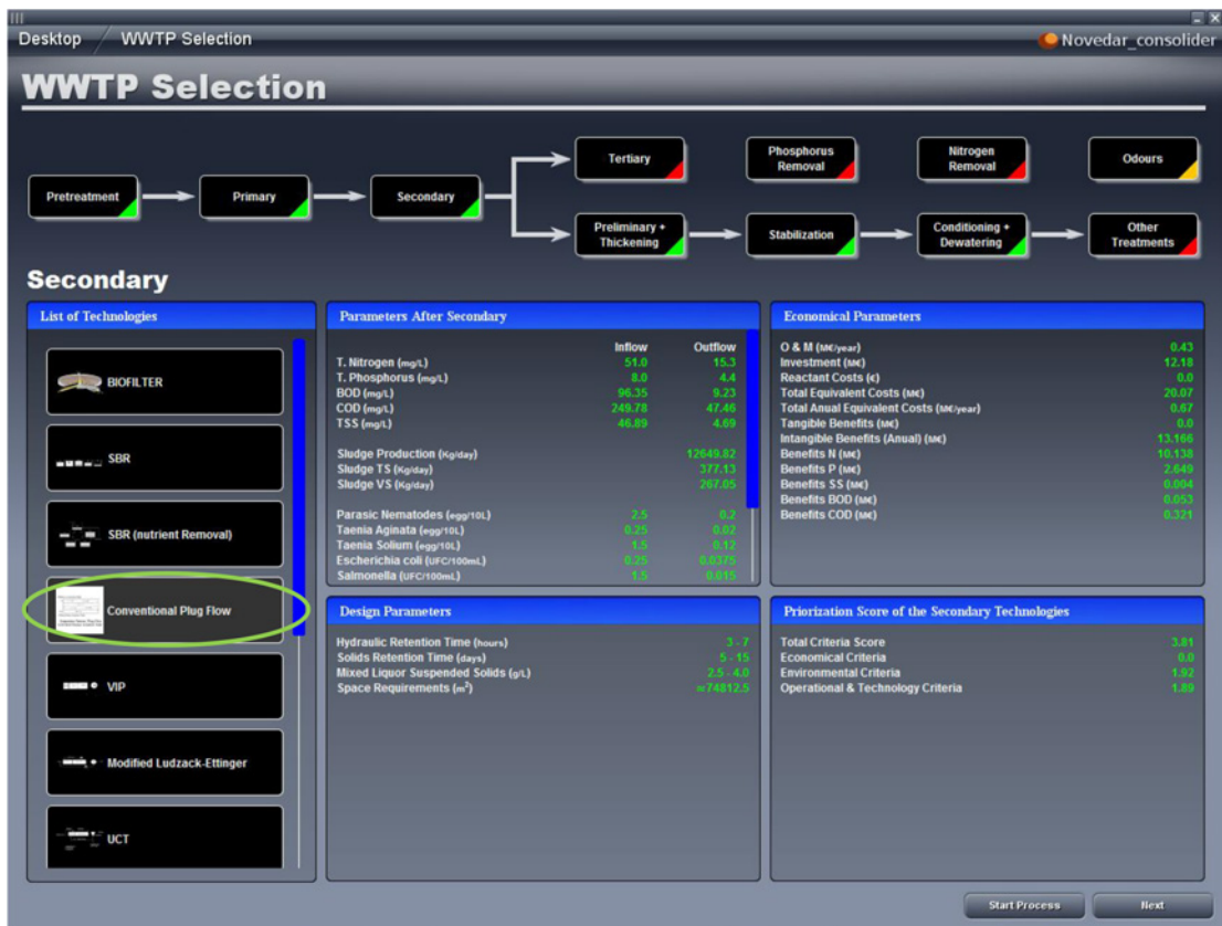
Figure 26.8 EDSS screen with the list of secondary treatment alternatives feasible for case study#2. They are scored based on economic, environmental and operational criteria.
