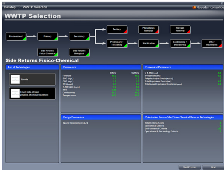
Figure A3.16 Snapshot of the generated treatments interface showing the physico-chemical treatments included in the side-stream as well as their score from the multi-criteria analysis.
