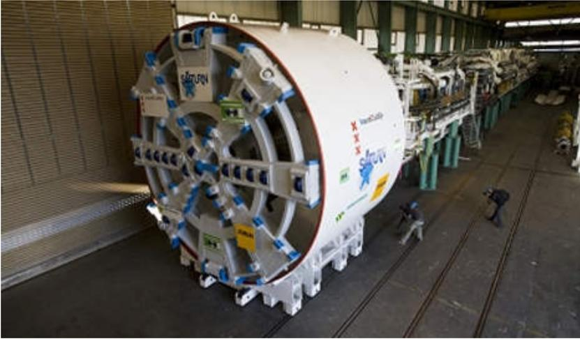
**Figure 4.1.** Drilling head of equipment used by Bouygues for the Amsterdam metro. (Source: AD, December 8, 2009.)
