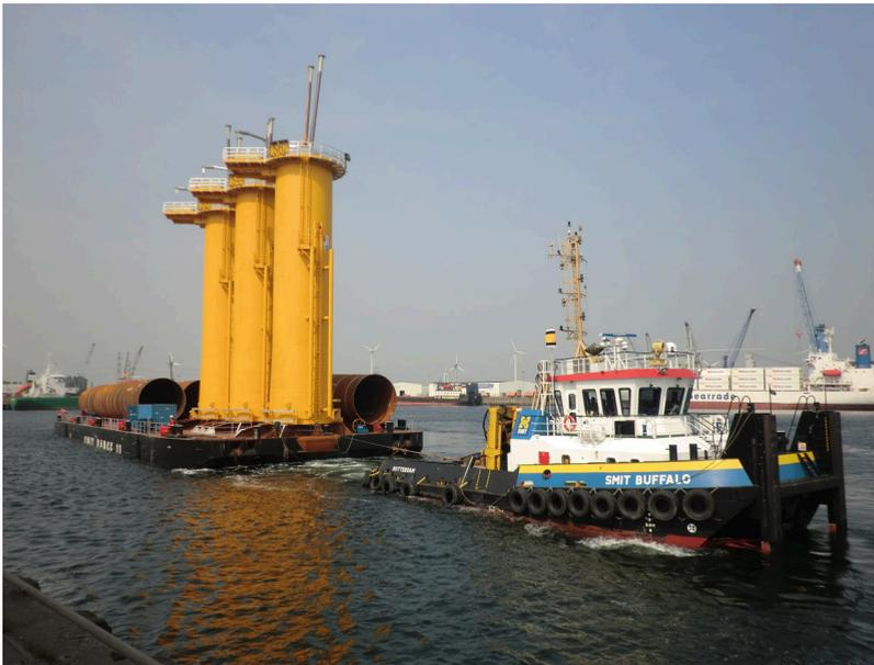
**Figure 19.2.** Sea transport of three wind turbine foundations with sub-piles for wind farm under construction. Best risk allocation is on a knock-for-knock basis. (Photo: SMIT, [www.smit.com/tugmagazine/june2011](http://www.smit.com/tugmagazine/june2011).)
