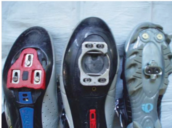
Fig. 22.8 Cleats attached to shoes outsole, left two shoes are external, right shoe is recessed
