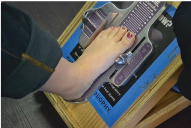
Fig. 6.1 Brannock Device shown being used for measuring foot metrics
