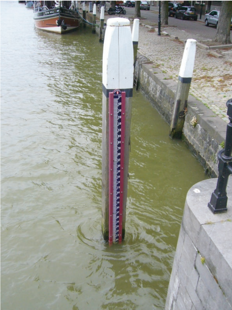
Fig. 4.1 Water level measurement in Dordrecht, the Netherlands
