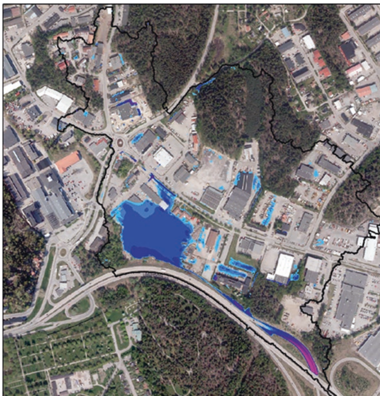
Fig. 10.2 Flood depth at a modeled pluvial flooding before preventive measures in Södertälje at the 1/100 – year event (flood depth varies from 0 to 3 m)
