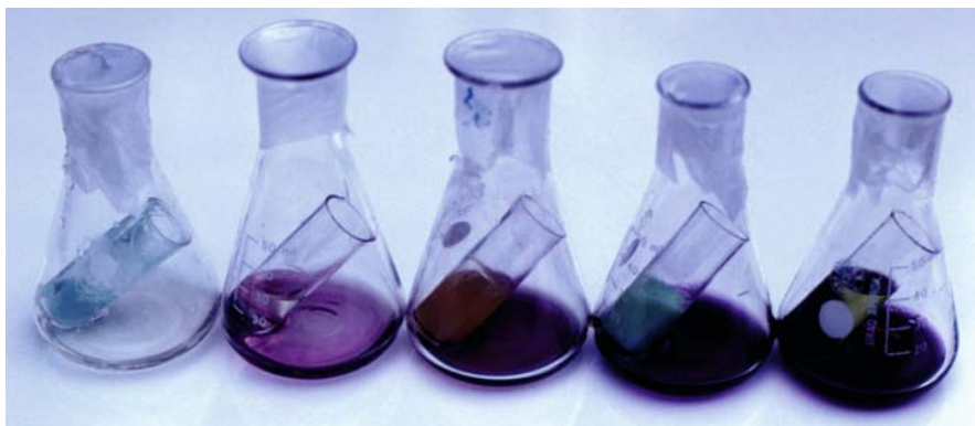
Fig. 7.10 Chromotropic acid spot test for formaldehyde in shampoos. Negative ( left ) and positive reactions (see explanations in text)
