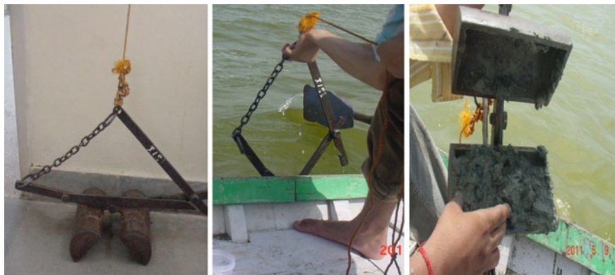
Photo 1 Peterson sediment sampler used for sediment sample collection from the Upper Lake, Bhopal
