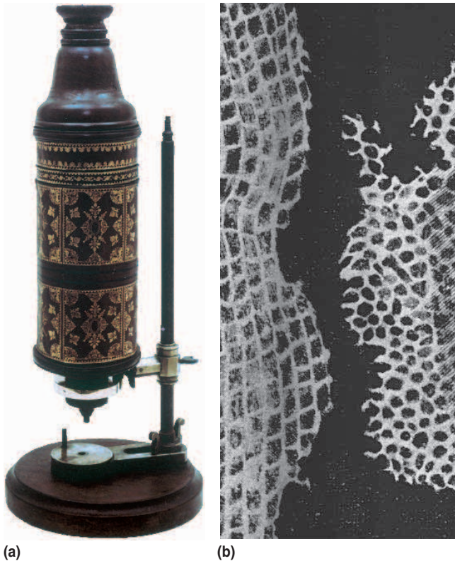
FIGURE 1.4 Hooke's Compound Microscope. (a) The compound microscope had a lens at each end of a tubular body. (b) Hooke's drawing of cork cells, showing the thick cell walls characteristic of plants.
