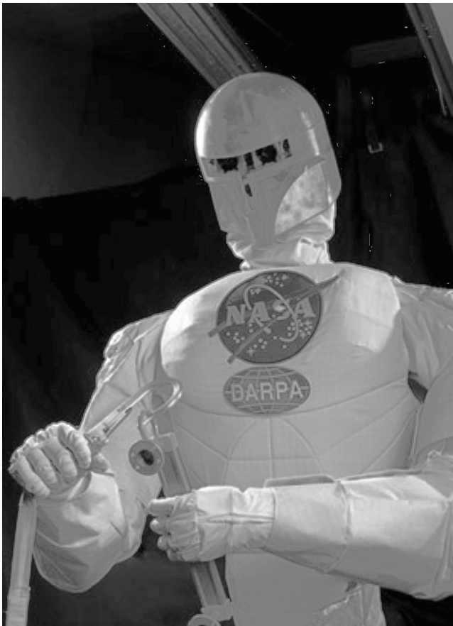
Figure 3.1 NASA and DARPA have developed Robonaut for work on the International Space Station. Robonaut has a dexterous five-fingered hand that can grasp and manipulate a wide variety of tools. Photo courtesy of NASA.
