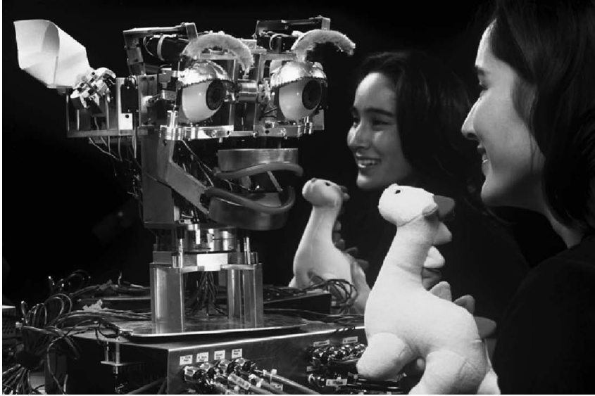
Figure 11.6 Kismet expresses surprise as Cynthia Breazeal shows it a children's toy. Kismet displays facial emotions in response to human interaction and built-in drive systems. It can display interest, surprise, happiness, disgust, anger, sadness, fear, fatigue, and calm. © Peter Menzel / Menzelphoto.com
