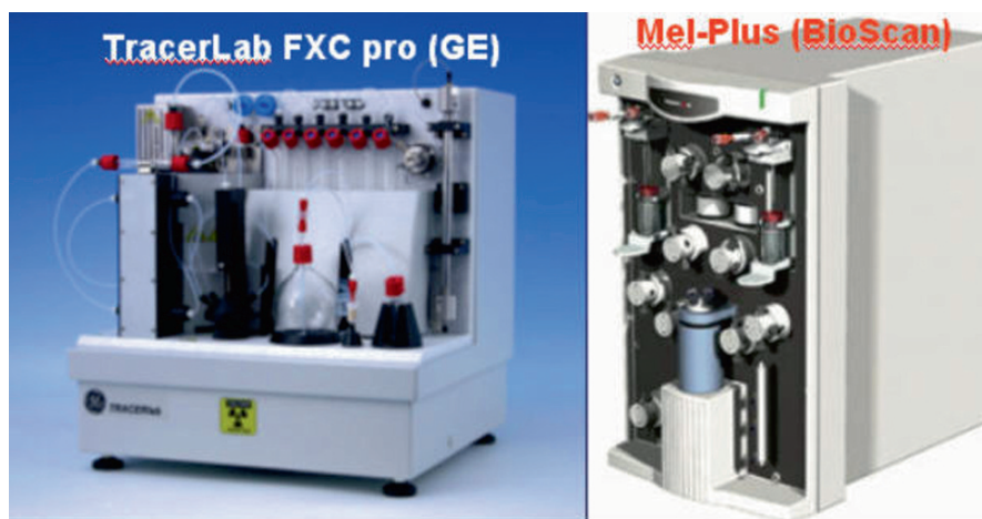
Fig. 11.4 Commercial automated synthesis modules for the production of ^{11}\text{C} Methyl iodide: TracerLab FXC pro based on gas phase method and MeI-plus based on liquid phase method
