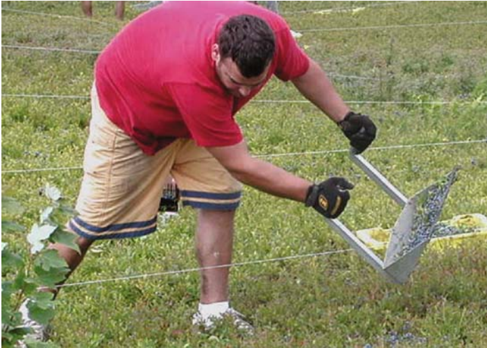
Fig. 4.5 A blueberry rake with 12-in. handle extensions
