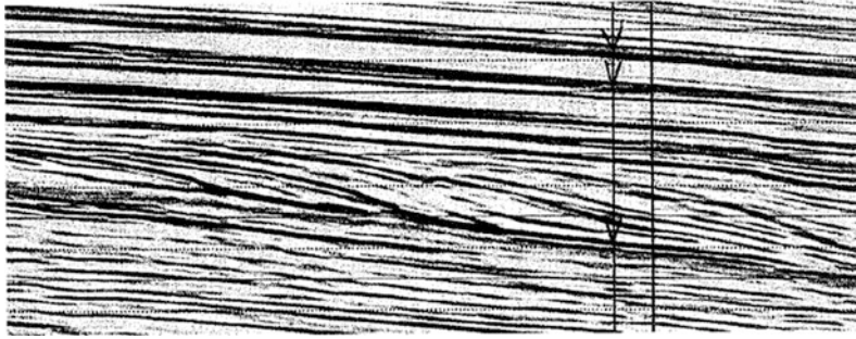
Fig. 11.63 Seismic reflection characteristics of river-dominated delta of continental shelf basin in north of the South China Sea
