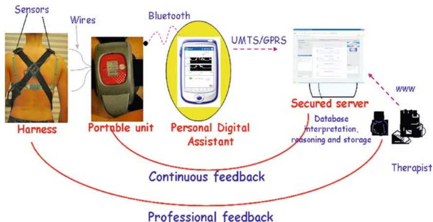
Fig. 36.2 Components, data transmission, and ways of feedback provision in the MYOTEL intervention.
