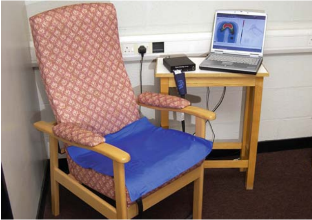
Fig. 7.1 The pressure mapping system.
