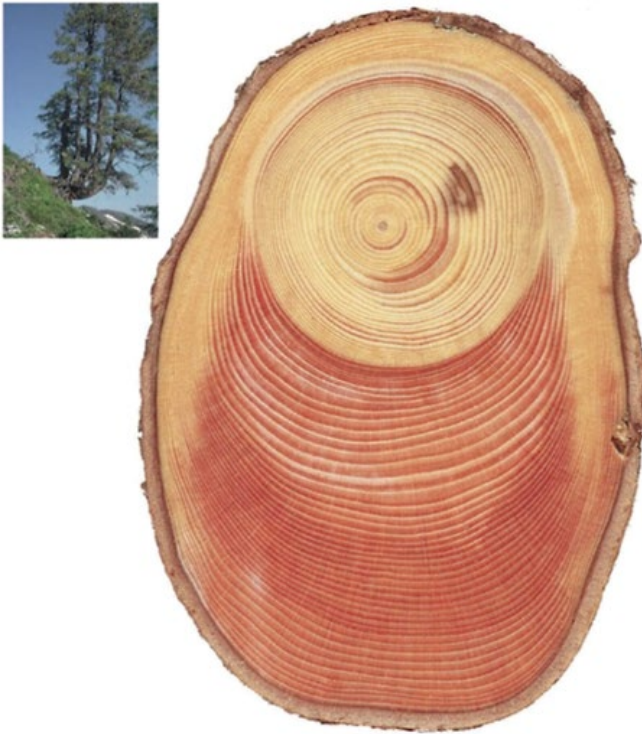
Figure 3.35 Reaction wood. Here, compression wood in a gymnosperm is seen as the darker portion on the lower side of this stem. If this was an angiosperm stem, the tension wood would be in the upper part of the stem. The inset illustrates how it is sometimes necessary to reorientate the crown to achieve vertical growth. Source: Schweingruber et al. (2006). Reproduced with permission of Springer.
