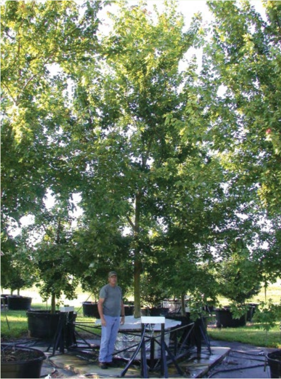
Figure EB4.1 Large suspension lysimeter used to measure the loss of water from the containerised tree. Source: Courtesy of Richard Beeson.
