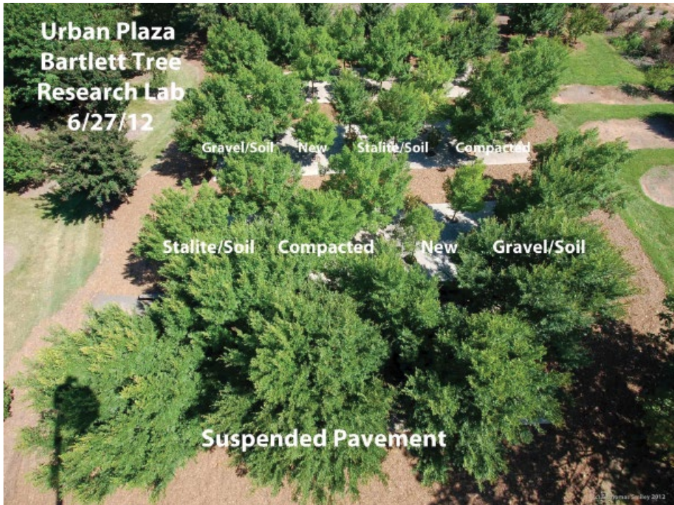
Figure 4.34 The Urban Tree Plaza experiment based at the Bartlett Tree Experts research laboratories in Charlotte, North Carolina, USA. Trees growing in the suspended pavement system that mimics the crate-based systems discussed in the text, out-performed those growing in structural soils (Stalite and Gravel) or compacted soil (Compacted). In lower image, 'New' represents replacement trees where the first planted tree has previously died. Source: Courtesy of Thomas Smiley.
