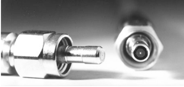
Fig. 8.3 A typical fiber connector. At the center of the ferrule, one can see the fiber either as a dark or a bright spot, depending on lighting conditions
