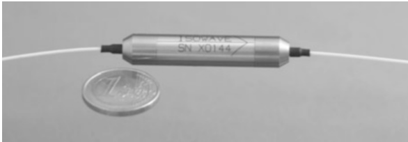
Fig. 8.12 An optical isolator. It comes with two fibers attached, known as “pigtailed”. The engraved arrow indicates the forward direction. A 1 Euro coin is shown for size comparison
