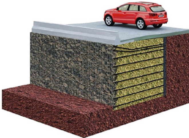
Fig. 1. 3D View of a GeoTrel ® Structure
