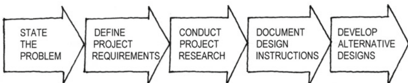
Figure 7-3. The six-step design process expressed as a linear sequence.
