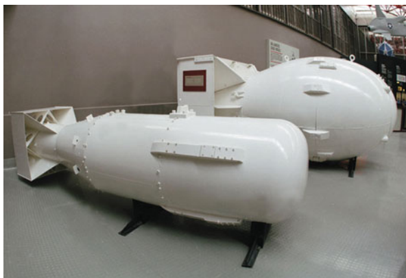
Fig. 4.17 American atomic bombs “Little Boy” (of gun type, with a blast equivalent of 15 kt of TNT, based on uranium-235) and “Fat Man” (of implosion type, based on plutonium-239, with a blast equivalent of 21 kt of TNT) dropped on the cities of Hiroshima and Nagasaki [8]
