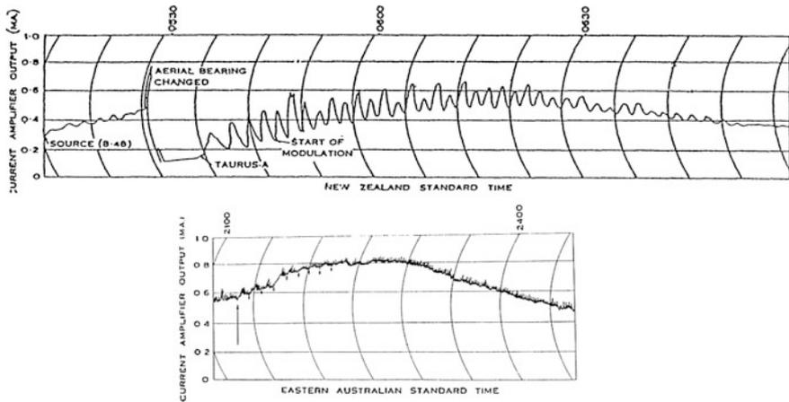
**Fig. 24.6** Chart records, to the same scale, showing the Taurus-A interference fringes as seen at Pakiri Hill, New Zealand (top) and Dover Heights (bottom) (after Bolton and Stanley 1949: 140–141)
