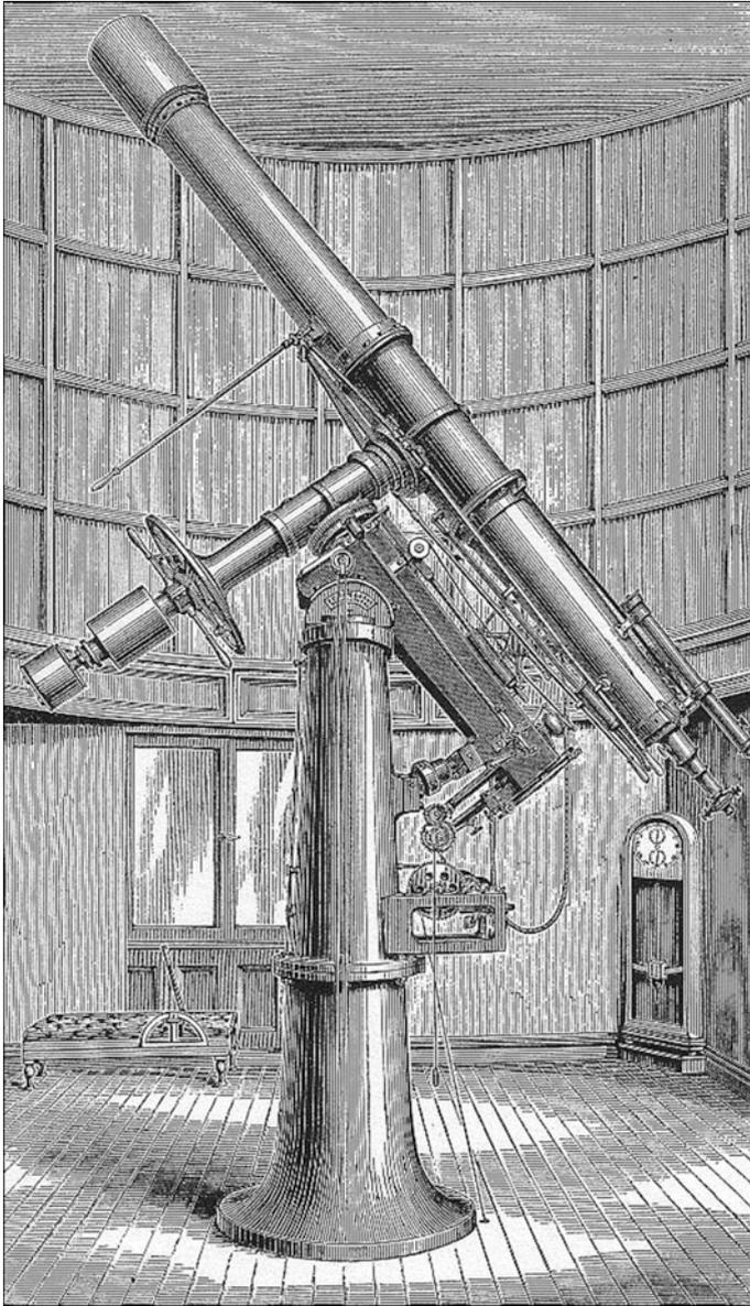
**Fig. 13.1** The 23.7-cm Cooke refractor (after Crossley et al. 1879: 10)
