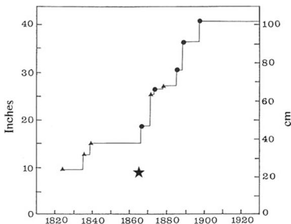
**Fig. 13.3** Plot of the way in which the aperture of the world’s largest refracting telescope changed during the nineteenth century. *Triangles* indicate Cooke telescopes and *circles* Alvan Clark telescopes. The Crossley refractor is represented by the *star*
