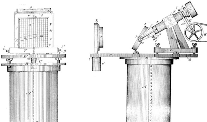
**Fig. 15.3** Details of the design of the horizontal photographic telescope, showing the plate-holder (left) and heliostat (right) (after Newcomb 1880)
