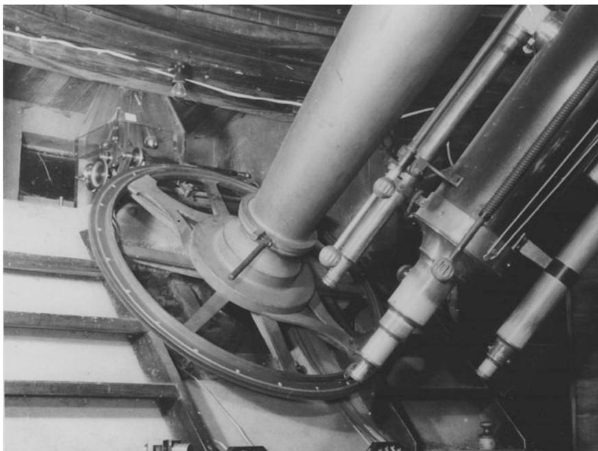
**Fig. 11.7** View of the lower end of the polar axis and main telescope tube (Orchiston collection)
