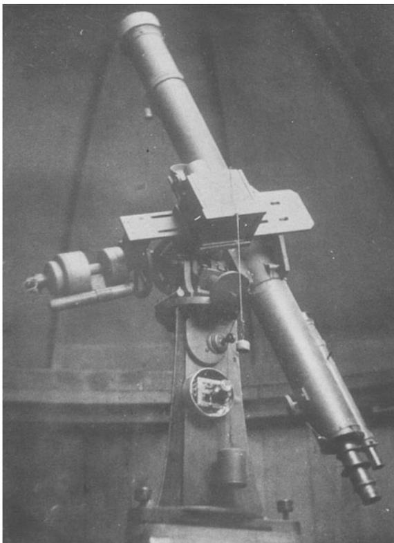
... an object glass of  $3\frac{1}{2}$  inches [8.9-cm] clear aperture, and a focal length of 54 inches [i.e.  $f/15$ ], with magnifying powers ranging from 60 to 480, sun prism, diagonal eyepiece, and other adjuncts necessary for the effective use of a first-class instrument. The equatorial mounting has a latitude arc and six-inch declination and right ascension circles ... (ibid.).
