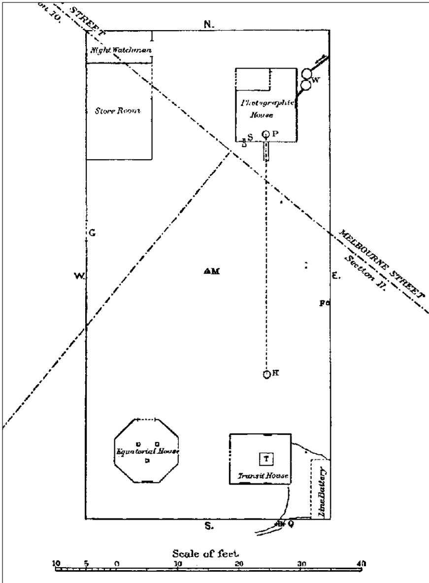
Fig. 15.11 Plan of Queenstown transit station. Key: T transit telescope; H heliostat; P photographic plate-holder (after Newcomb 1880)
