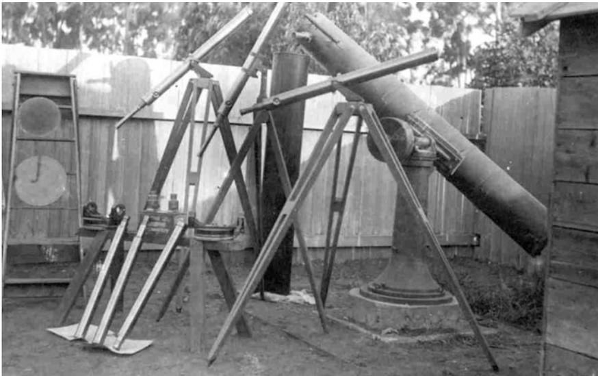
**Fig. 12.6** An assortment of small refractors and a reflector made by Ward (*Courtesy Ward (Wanganui) Observatory Archives*)
