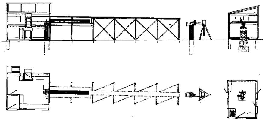
**Fig. 15.4** The overall arrangement of the horizontal photographic telescope and 'Transit House'. Top side elevation; bottom plan (after Orchiston et al. 2000: 27)
