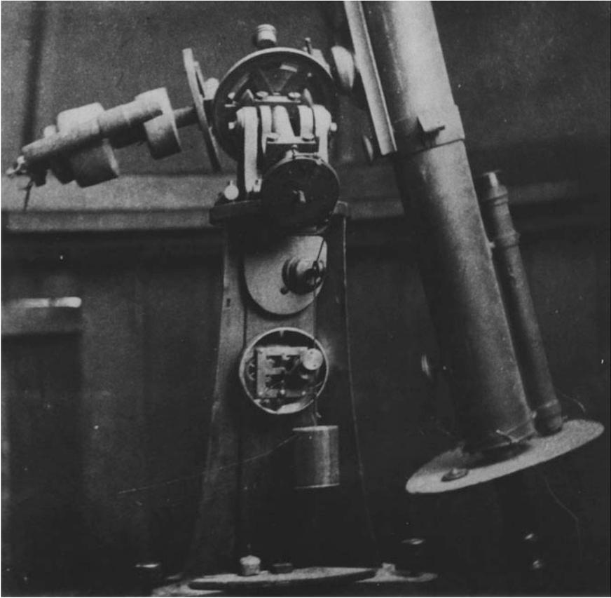
**Fig. 10.4** A close-up view of the home-made equatorial mounting and drive (*Courtesy Ward (Wanganui) Observatory Archives*)
