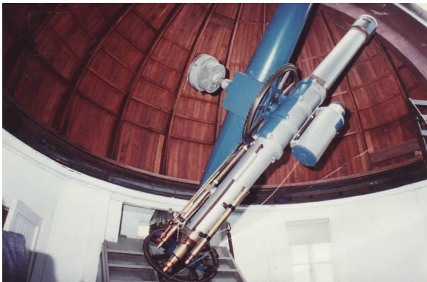
**Fig. 11.10** A 1999 photograph of the 24.1-cm (9.5-in) Cooke refractor and 22.8-cm (9-in) Houghton-Rumsey Astrograph, along with the main telescope's distinctive English equatorial mounting (Orchiston collection)
