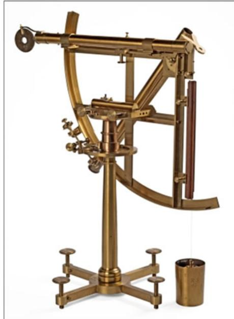
used by Cook for observing the transit of Venus at Tahiti.” Both of the telescopes have 1.9-cm objectives of 33cm focal length, and the eyepiece end of the lower telescope is “... fitted with verniers, clamping screw and slow motion which traverses the limb which is divided into two scales one into  $90^\circ$  and the other  $96^\circ$ , according to Bird’s method, each reading to  $1'$  of arc ...” (Science Museum catalogue entry). Figure 4.17 shows one of these instruments.
