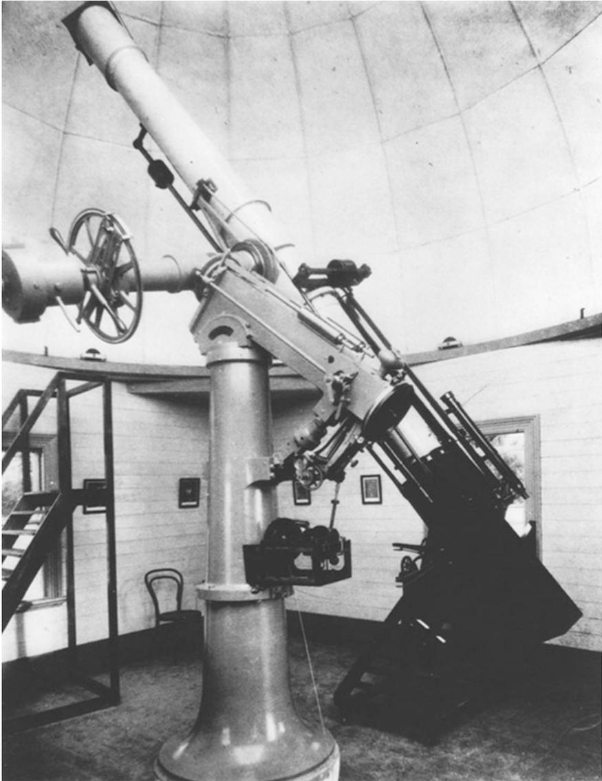
**Fig. 22.17** The 23-cm (9-in) Cooke photovisual refractor at the Meeanee Observatory (Orchiston collection)
