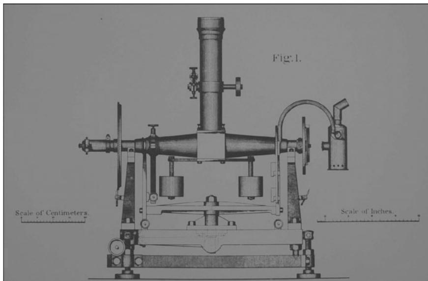
**Fig. 15.6** A schematic of the Stackpole ‘broken tube’ transit telescope (after Orchiston et al. 2000: 28)
