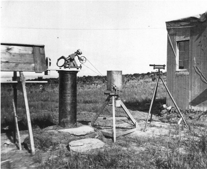
**Fig. 14.11** The Chatham Islands horizontal telescope showing (left to right) the protective wooden framework (leading to the ‘Photographic House’), the heliostat and pier, the heliostat weight drive, an engineer’s level, and part of the ‘Transit House’ (Courtesy Alexander Turnbull Library, Wellington, Ref. PAColl-0058-02)
