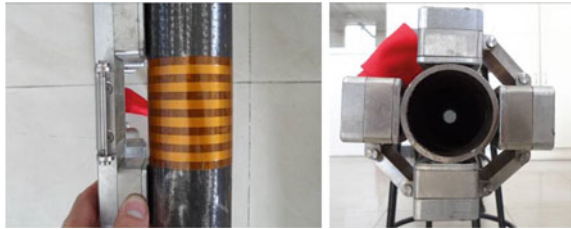
Fig. 7.11 A magnet made by the neodymium–iron–boron permanent magnet
