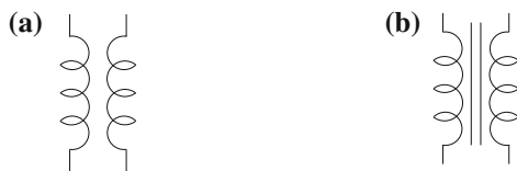
Fig. 6.12 Symbols representing static transformers: a air core transformer, b ferromagnetic core transformer
