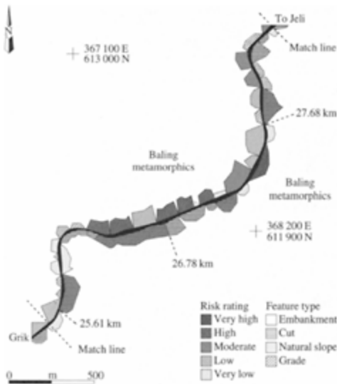
Figure 6.4. Typical risk map for a section of the East-West Highway study in Malaysia (Lloyd et al. 2001).
