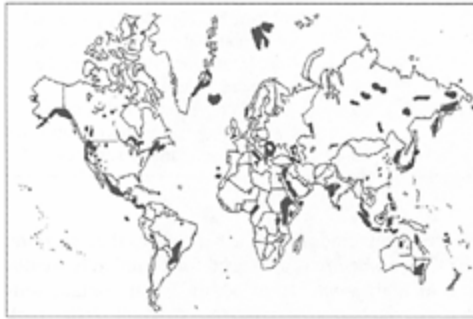
Figure 1.14. (c) Residual soils developed from extrusive igneous rocks, primary basaltic plateaus and mountains (Rollings & Rollings 1996).
