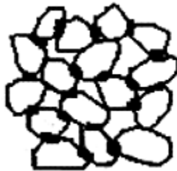
Figure 9.3. Cementation effect around the contact points of coarse grains (Kezdi 1979).
