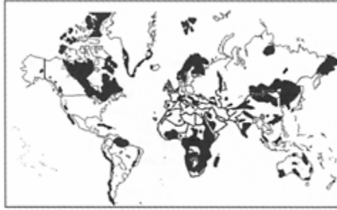
Figure 1.14. (b) Residual soils developed from intrusive igneous rocks, primary granitic shields and mountains (Rollings & Rollings 1996).
