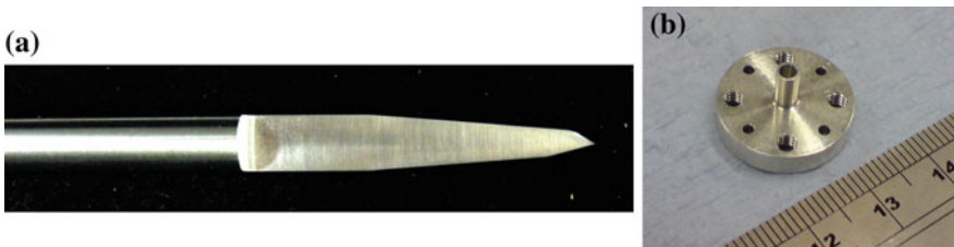
Fig. 2.4 a The high speed steel machine tool used to fabricate the multiple flare-angle horns. b A prototype of 700 GHz smooth-walled horn made by direct milling into an aluminium block
