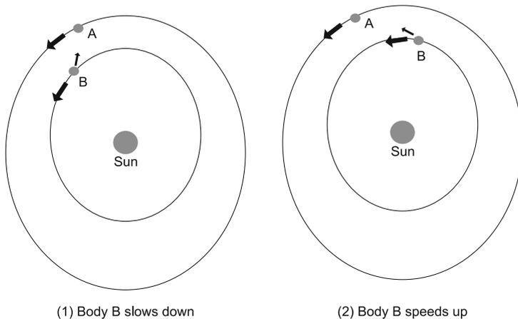
**Fig. 1.4** An example on the effects of orbital resonances of two objects
