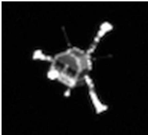
**Fig. 6.13** This image shows the Philae lander at 10:23 GMT on 12 November. The image shows details of the lander, including the deployment of the three legs and of the antennas (credit: ESA/Rosetta/MPS for OSIRIS Team MPS/UPD/LAM/IAA/SSO/INTA/UPM/DASP/IDA)
