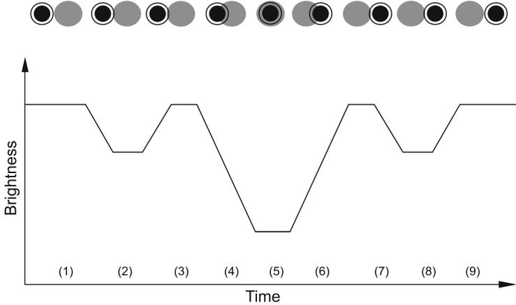
**Fig. 6.3** Basic principle of how to detect a ring system around a body using stellar occultations
