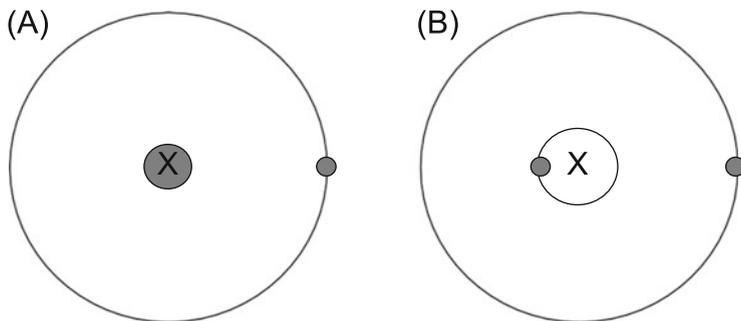
**Fig. 5.2** Illustration of the barycenter (center of mass) in two scenarios: (a) the primary object in the center has a clearly dominant mass compared to the orbiting moon. Hence the barycenter lies close to the central objects core; (b) differences in masses of primary object and moon is lower. The barycenter lies outside of the primary object (similar to the Pluto-Charon system)
