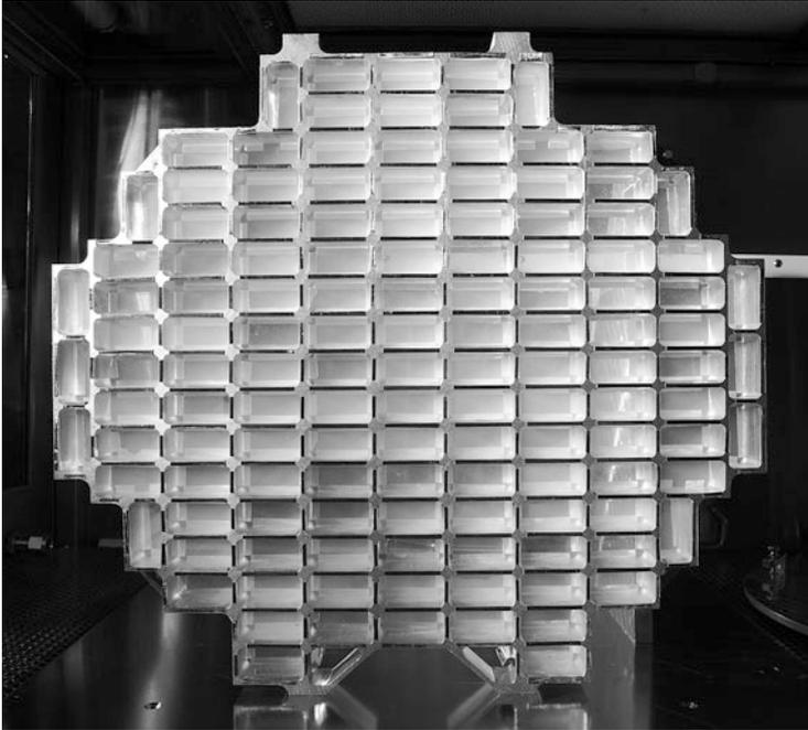
**Fig. 6.25** Stardust Dust Collector with aerogel (credit: NASA/JPL)
