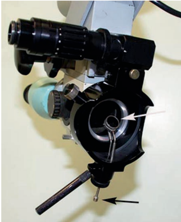
Fig. 10.7. Joystick ( black arrow ) and movable mirror ( white arrow )
