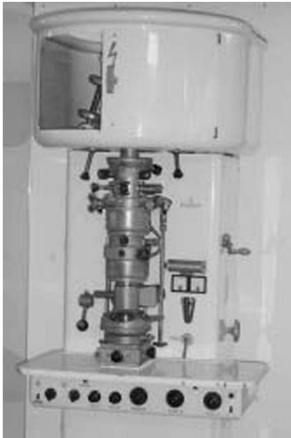
After only three years of development, in terms of its spatial resolution the electron microscope had outpaced the light microscope. Starting in 1939, an initial series of the Supermicroscope (“Übermikroskop”), as it was called at the time, was offered for sale by Siemens.
