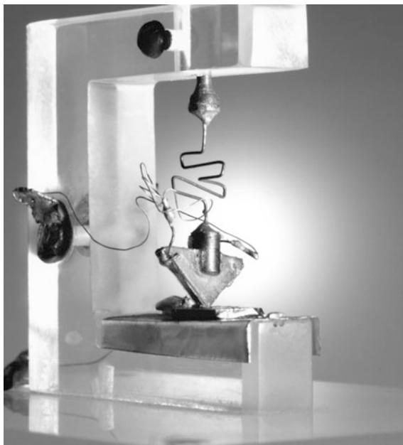
**Fig. 6.9** The first point-contact transistor constructed by Bardeen and Brattain in December of 1947. The three-cornered part in the *middle* is made from plastic material and is covered by a gold foil at its two edges. At the *tip* at the *bottom* the gold foil is cut by a razor blade, such that two contacts are generated in close proximity. By means of a metal spring the contacts are pressed against the semiconductor surface located underneath (*Photo Lucent*)
