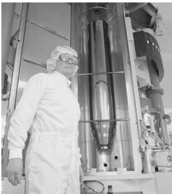
heating zone is slowly moved from one end of the crystal to the other. In the resulting temperature gradient the atomic impurities are carried along to one end of the crystal. If necessary, this process can be repeated several times. The impurity concentration of silicon single crystals, routinely achieved today in the semiconductor industry, amounts to only about a single impurity atom within 1 billion silicon atoms.
