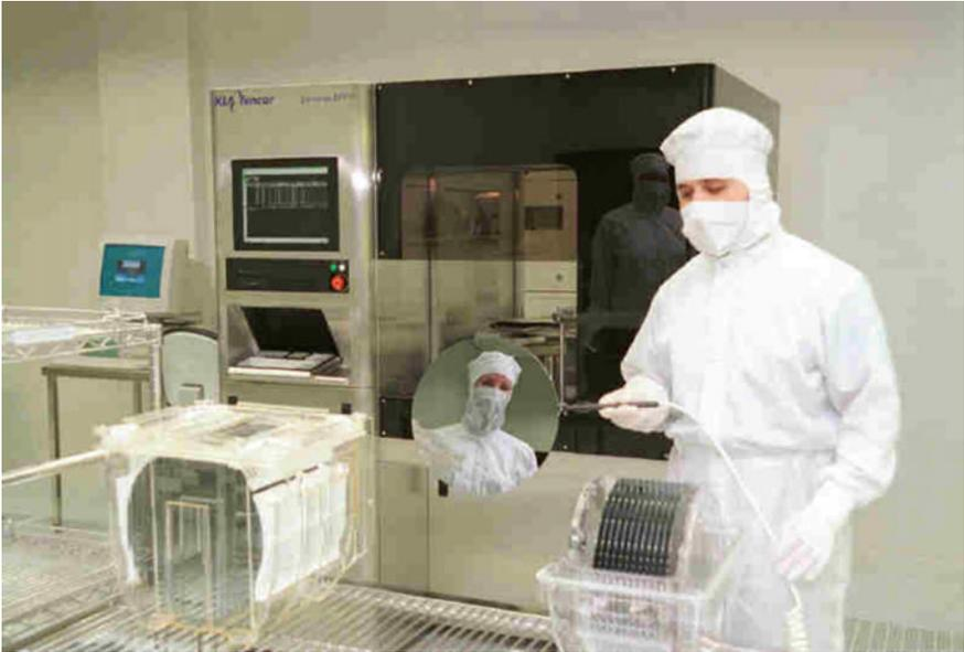
**Fig. 6.11** Processing of the silicon wafers with 30 cm diameter (*Photo Wacker Chemie AG*)
