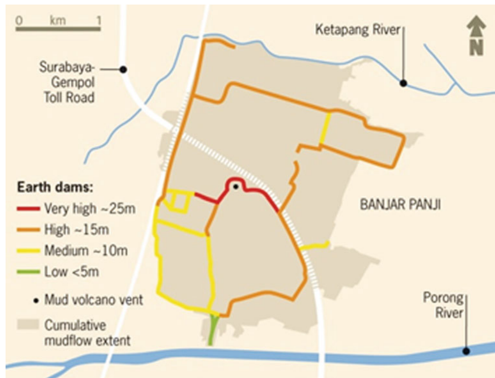
Fig. 21 Construction of permanent dykes (BPLS 2007)
