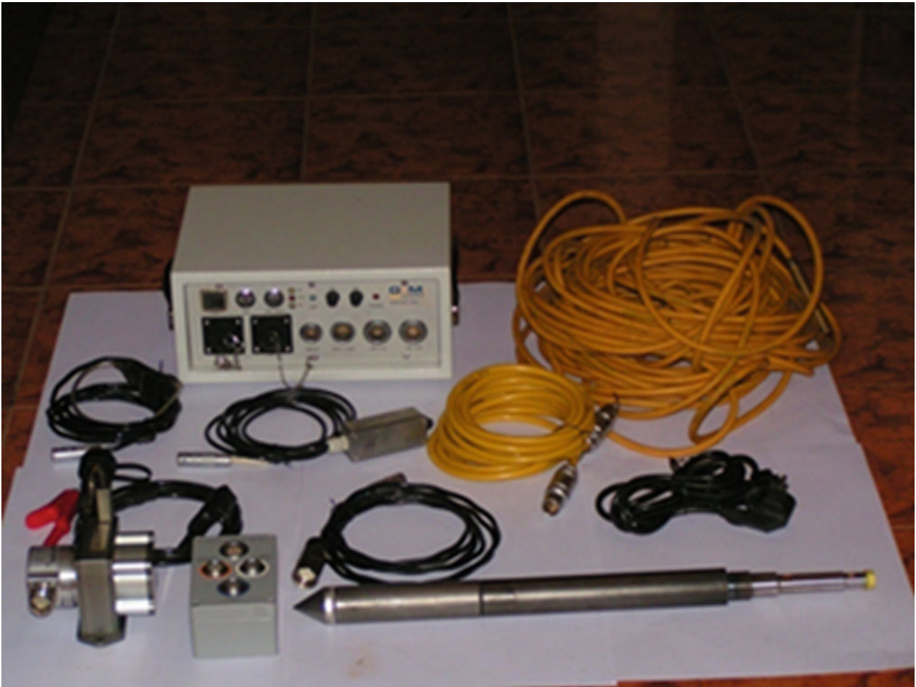
Fig. 13 CPTu equipment for the research of lusi
