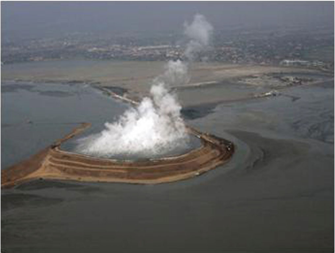
Fig. 2 The vent of the mud eruption in East Java, Indonesia, surrounded by protection dykes (Boston.com 2008)
