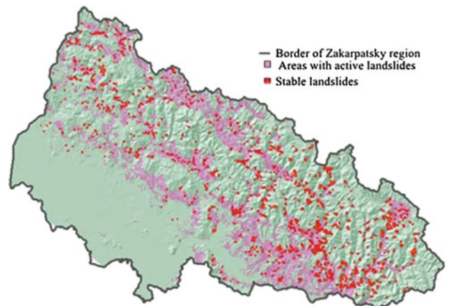
Fig. 5 Remote sensing data on the distribution of landslides sites within the Zakarpatsky region
