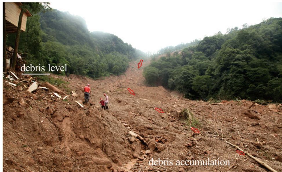
Fig. 3 The debris flow, showing the height difference of about 15 m between the maximum level and the accumulation
