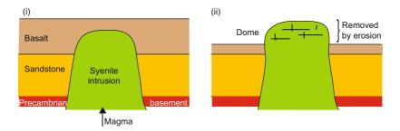
**Fig. 11.4** Formation of the syenite domes at Axum. (i) Magma intrudes through the overlying rocks but solidifies before it reaches the surface. (ii) The overlying rock is eroded, revealing the top of the dome and releasing pressure on it so that the rock expands a little and cracks, producing elongated slabs separated by weaker joints
