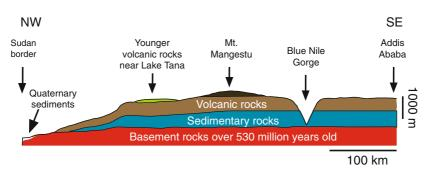
**Fig. 4.3** A schematic geological cross section through the Western Highlands, along the *dashed line* shown in Fig. 4.2. Note that the vertical scale is greatly exaggerated
