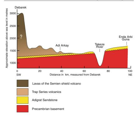
**Fig. 9.3** Geological cross section through the Tekeze Gorge between Debarek and Enda Arbi Guna. The *question mark* indicates uncertainty as to where the boundary is between the lava flows of the Trap Series, and those of the Semien shield volcano
