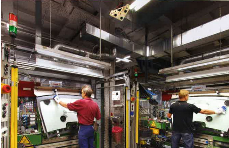
Fig. 13.5 The SAFETYEYE two-axis stereo camera with three HDRC sensors monitoring the safe operations of two operators in the man-machine directed assembly of wind-shields for automobiles [11]
