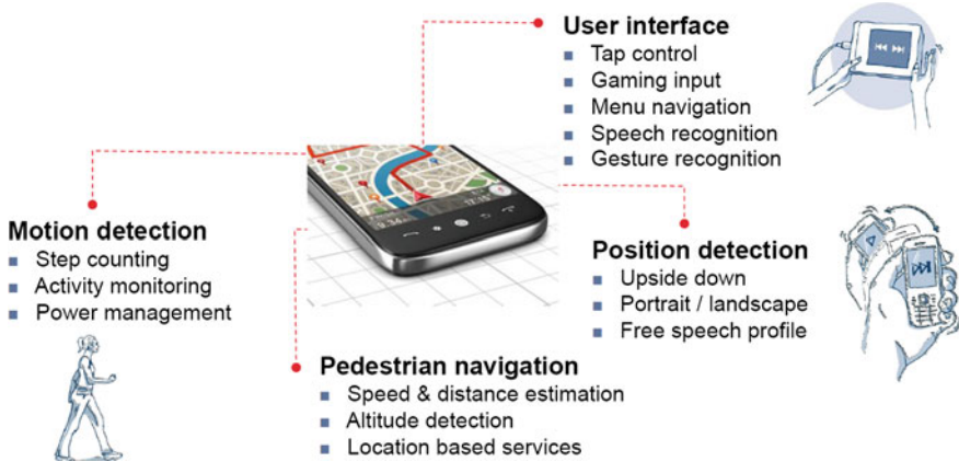
Fig. 15.11 MEMS enable intuitive and realistic implementations of human-machine interfaces
