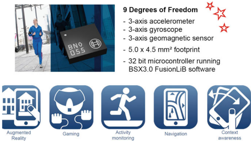
Fig. 15.13 Absolute-orientation sensor, 5.2 × 3.8 mm 2 . Integrated system with 9 degrees-of-freedom [3]
