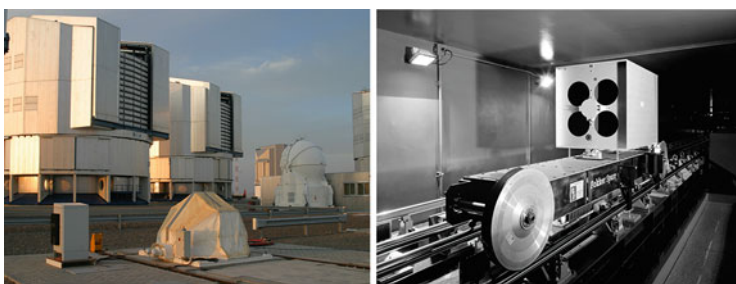
Fig. 6.1 Left : Light collectors used for the observations of Achernar: 0.4m test siderostat ( foreground ), 1.8m auxiliary telescopes ( right ) and 8.2m unit telescopes ( background ). Right : One of the long delay lines of the VLTI
