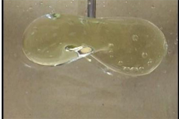
Fig. 9.11 Experiments with rotating drops of castor oil: peanut shape. Photo courtesy of the ACE-REU Program, Georgia Institute of Technology
