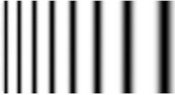
Fig. 2.38 Spatial chirp generated by a density plot of a function \sin^8 [(1 + x)x] , with a linear increase in frequency from right to left . The illusion of wider patterns being closer persists
