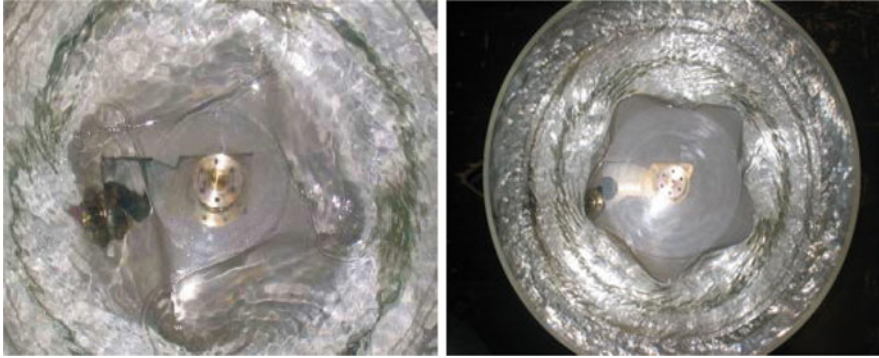
Fig. 9.32 Experiments with a rotated water column contained in a cylinder, viewed from the top . Left : Squares with Görtler vortices spiraling at the corners. Right : Pentagons. Regular polygons with 3–6 edges form spontaneously because of the instability of the inner fluid surface. The number of edges depends on the height, radius, and angular frequency: the shallower the cylinder and the faster it is rotated, the more edges are generated. Courtesy of Phys. Rev. Lett. 96 (2006)
