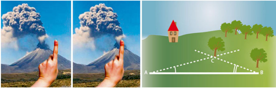
Fig. 3.3 Left: The parallax of your own finger: seen from your left eye you see the finger in a different direction with respect to the background than seen from your right eye. Right: The distances to the remote tree C from the points A and B, respectively, are AC and BC. These distances can be calculated by measuring at A the angle CAB between the directions to B and C, and at B the angle ABC between the directions to A and C, and then measuring the distance AB between A and B. Now two angles and one side (AB) of the triangle ABC are known and AC and BC can be calculated. This is the way in which prospectors measure distances to remote objects
