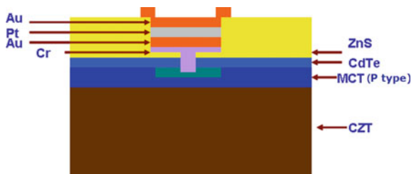
Fig. 5.59 Schematic diagram of the electrode in the HgCdTe device
