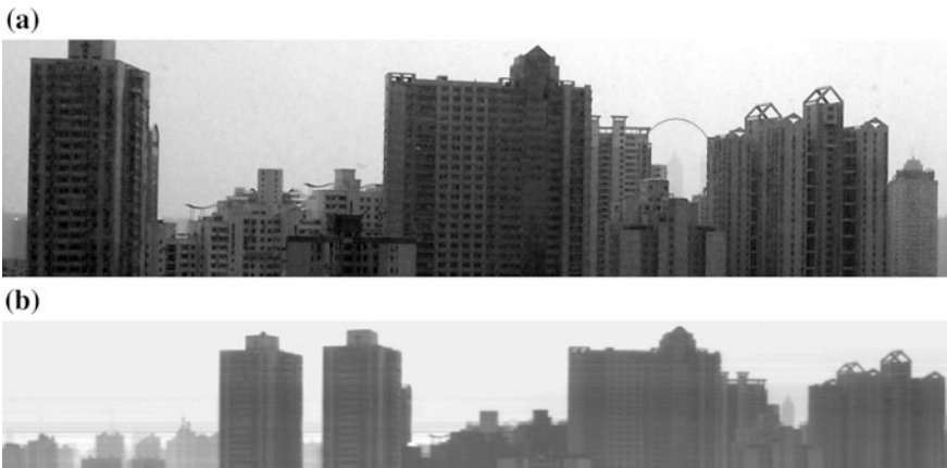
Fig. 6.113 Experimental results of long distant scene imaging a gray photograph of visible light imaging, b photograph of visible-blind waveband imaging
