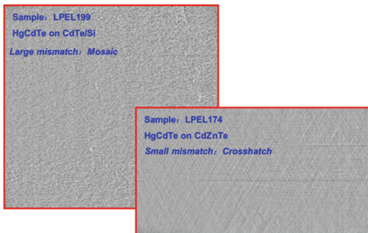
Fig. 3.103 X-ray diffraction morphology of Si-based LPE film
