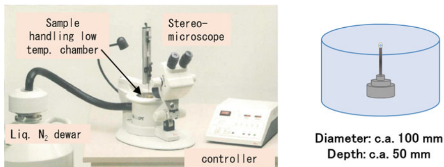
Fig. 9.7 Low-temperature sample handling tool, EM CPC: overview (left) and sample chamber schematic view (right), here one can handle cooled sample in cool nitrogen air in the chamber with stereomicroscope
