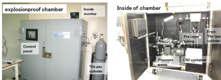
Fig. 9.6 High-pressure freezing machine, HPC-201: outside view (left) and inside view (right)
