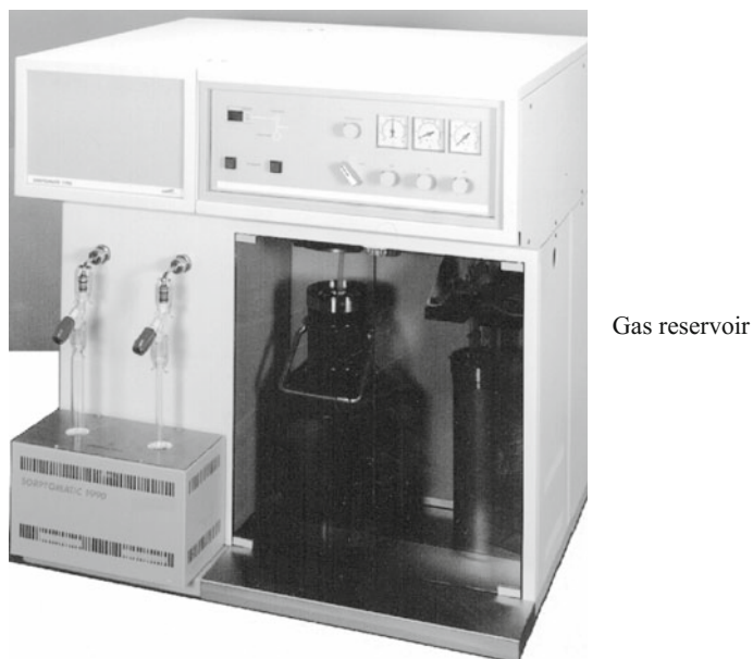
Fig. 3.14 An automatic gas-volumetric commercial apparatus for measuring nitrogen adsorption at 77 K (Instruction manual of Sorptomatic)
