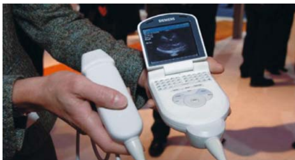
Fig. 19.3 Miniature handheld echocardiographic machine
