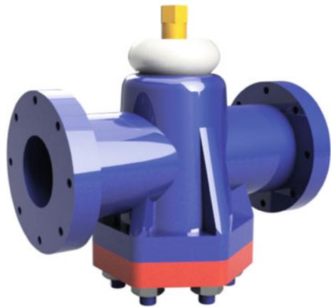
The wheel regulates the gap between the plug and the body. The valve works only with lubrication. The lubricant seals the valve and the thread of spindle, makes the turn of plug easier, and also prevents corrosion of details. The lubricant is supplied through the channel in the spindle with the pressure screw t, and then through the check valve inside the body.
