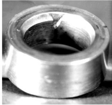
**Fig. 7.4** The fractured surface of the sucker rod pump valve
