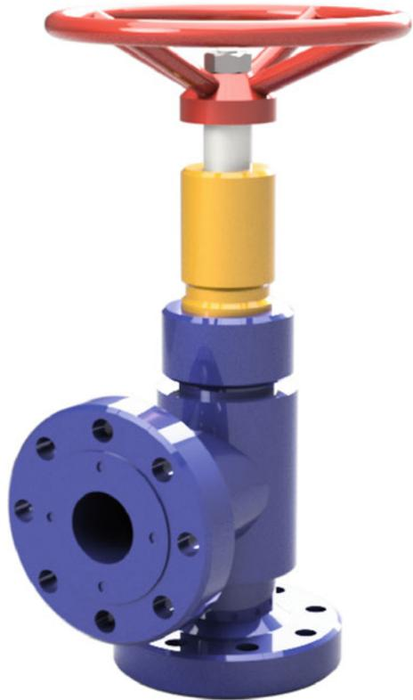
adjustable throttle with nominal diameters 65 mm, with working pressure 35 MPa, for fluids containing up to 6 % CO<sub>2</sub>, is written as DR-65×350K1/ДР-65×350K1.
