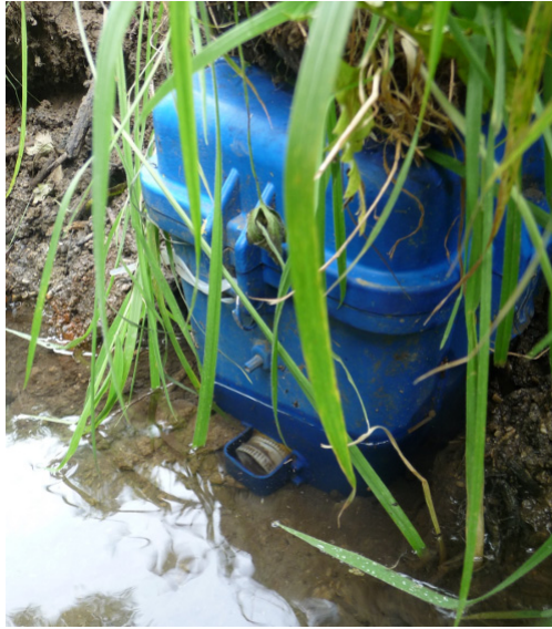
Fig. 7. The phosphate sensor in-situ during a trial at Broadmeadow Water, Co. Dublin, Ireland in September 2009. The sample inlet is visible below the water line.
