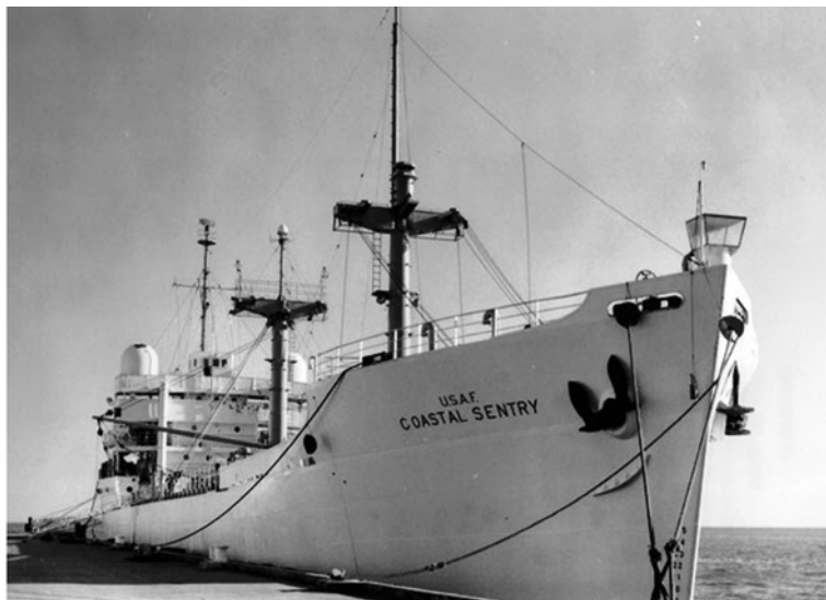
The USAF Missile Range Instrumentation ship Coastal Sentry (call sign Coastal Sentry Quebec ) was used as a communication station for MA-7 while stationed off the south-eastern coast of Africa. (Photo: USAF)
