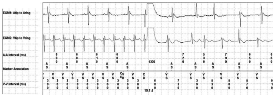
Fig. 2. Stored electrogram of a shock-terminated rapid ventricular tachycardia. Top tracing represents atrial electrogram, second tracing represents ventricular electrogram. Marker annotation describes device-defined event; “AS,” atrial sensed event; “VS,” ventricular sensed event; “CD,” charge delivered.
