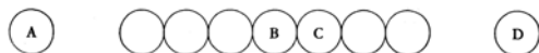
Fig. 14.3 A row of equal spheres of hard matter struck simultaneously from both ends.—[K.K.]
