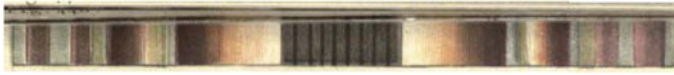
Fig. 20.7 The external fringes seen on each side of the shadow of a hair or wire, which is also divided by its internal fringes. The dotted lines show the natural magnitude of the shadow, independently of diffraction
