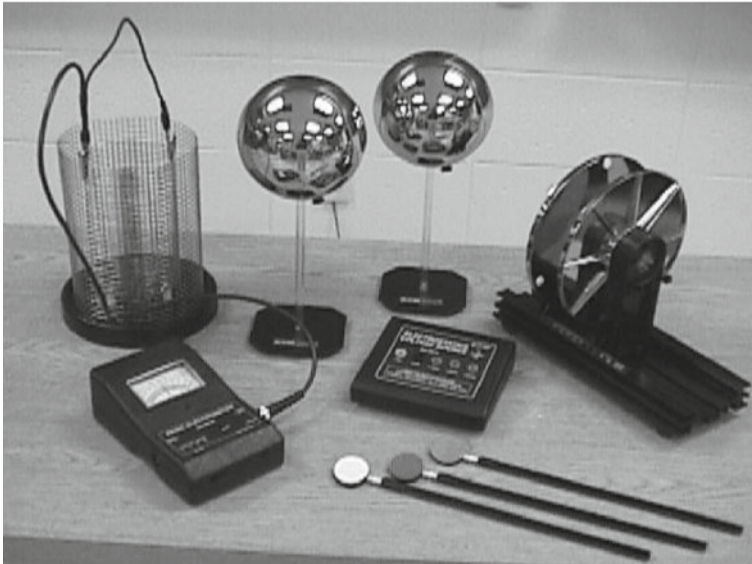
Fig. 4.4 Electrostatics equipment consisting of two conductive spheres ( top ), a volt power supply ( middle ), parallel-plate capacitor ( right ), charge producers and proof plane ( bottom ), and an electrometer wired to a faraday ice pail ( left )
