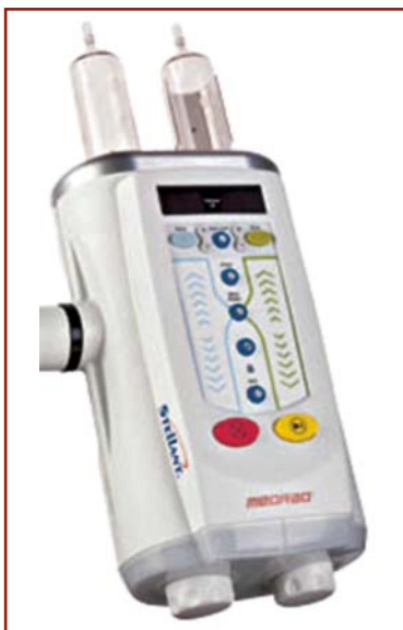
Fig. 3.3. Contrast-agent power injector (Stellant D, MEDRAD INC., USA), with permission
