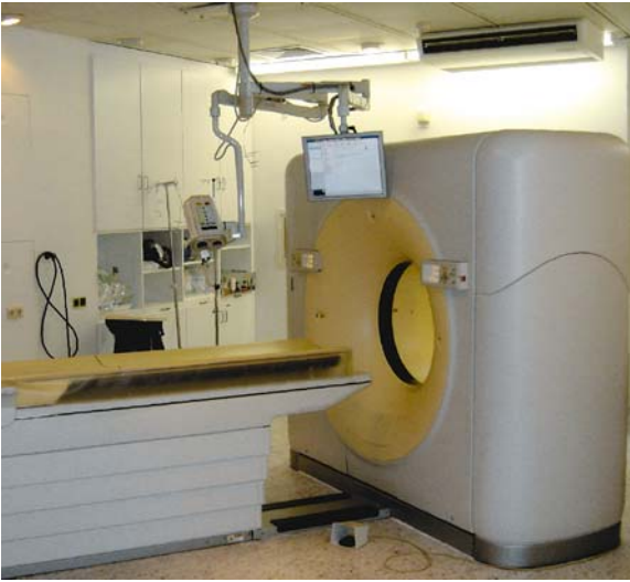
Fig. 2.4 A typical CT scanner room suitable for CT interventions equipped with a 64-slice CT scanner with a foot pedal, a monitor, and the option to perform fluoroscopic interventions
