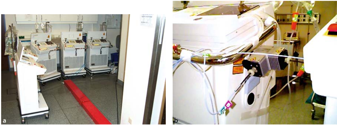
Fig. 13.29 a The setup of five laser systems (Dornier MediLas 5100) in the control room for simultaneous treatment of multiple lesions. To each of the five laser systems up to two laser fibers
