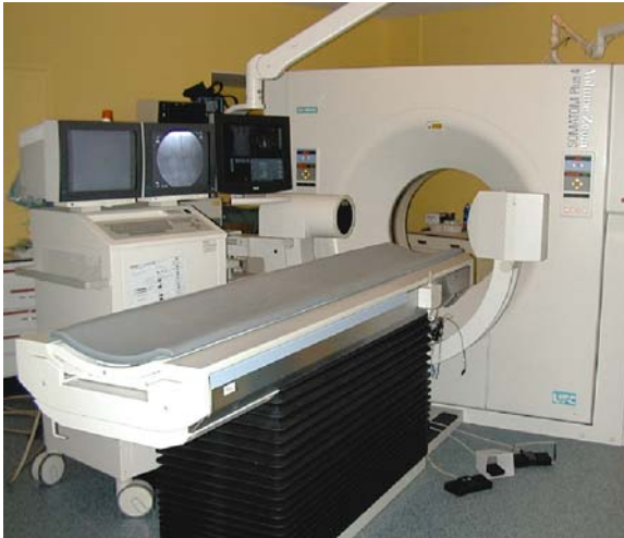
Fig. 15.7 Combined CT and mobile C-arm fluoroscopy setup for percutaneous vertebroplasty: CT guidance is used to choose puncture site and for needle placement while cement injection is performed under fluoroscopy control. This arrangement is preferred in the treatment of cervical or high thoracic vertebrae and sacroplasty where fluoroscopy alone is inadequate to visualize critical structures
