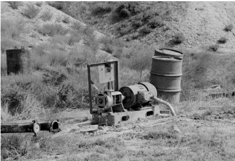
Photograph 4 , Mechanism used to pump Samine at the Alyat depot. The pump is no longer functioning and can probably not be repaired. A replacement pump would be necessary.
