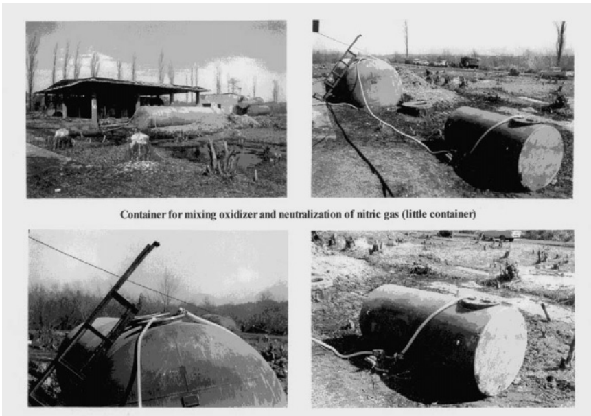
Figure 3, Container for mixing oxidizers and neutralization of nitric gas (little container)
