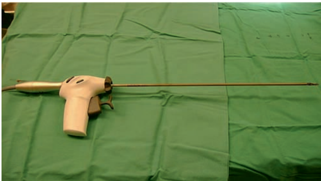
FIG. 8.2. Hand Piece and Blade. Gross photos of the hand piece containing a transducer that converts electrical energy to mechanical energy and transfers this energy to the distal blade
