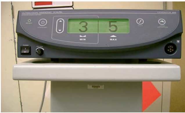
FIG. 8.1. Harmonic Scalpel Generator. The microprocessor-controlled generator utilizes AC current to pulse the transducer (Fig. 8.2) with electrical energy. The generator alters the power delivered based on microprocessors in the device. Note the LED screen demonstrating power settings (level 1–5)
