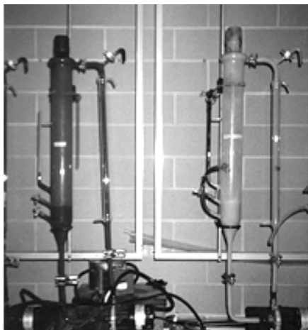
Fig. 5.2. Cyclone fermenters used for maintenance of hydrocarbon-degrading microorganisms
