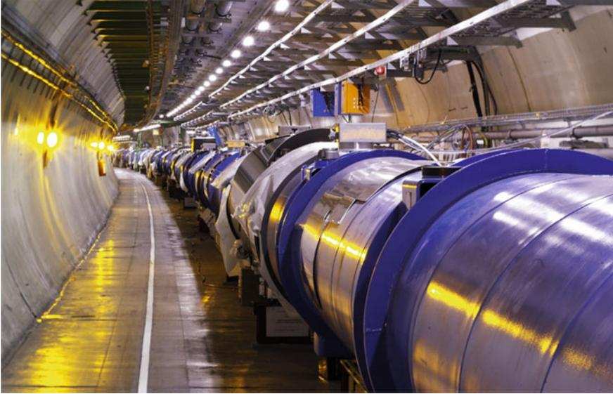
**Fig. 3.2** Real photo of the the superconducting magnets surrounding the beam pipe which hosts the LHC colliding protons [8]. The picture was taken before the start of the accelerating operations
