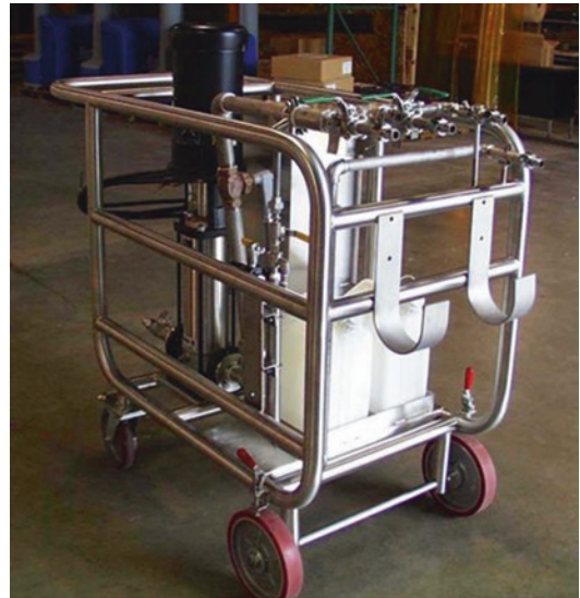
Fig. 11.1 A portable high-pressure, low-volume unit that is used where a centralized system does not exist. This unit is equipped with racks for hoses, foamer, and cleaning compound storage and provides two rinse stations and a sanitizer unit. Two workers can simultaneously pre-rinse, clean, post-rinse, and sanitize. This equipment can also apply foam if the spray wand is replaced with a foam wand accessory (Courtesy of Ecolab, Inc., St. Paul, Minnesota)
