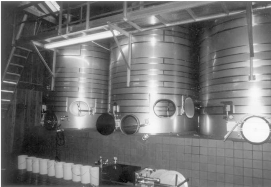
Fig. 20.1 Red wine fermentation tanks (Courtesy of Bruce Zoecklein, Virginia Polytechnic Institute & State University, Blacksburg, Virginia)
